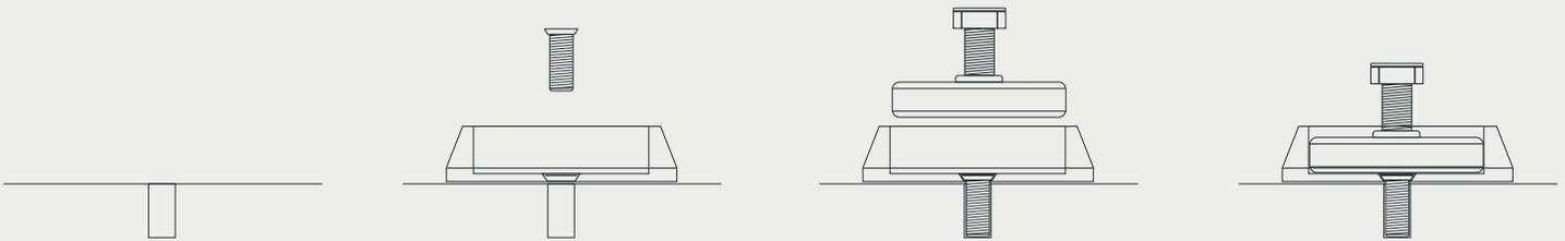
1. A pilot hole is drilled and a tapped metal plug is fixed in the deck.
